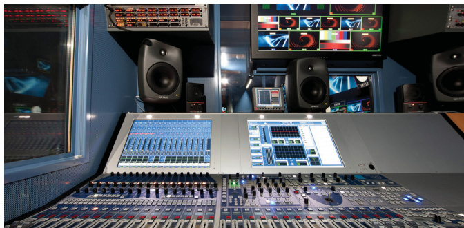
Evertz monitors and Grass Valley Kayak switcher feature in the truck's gallery, and the Lawo MC256 digital mixer, expandable to 48 faders, specified by ERR
