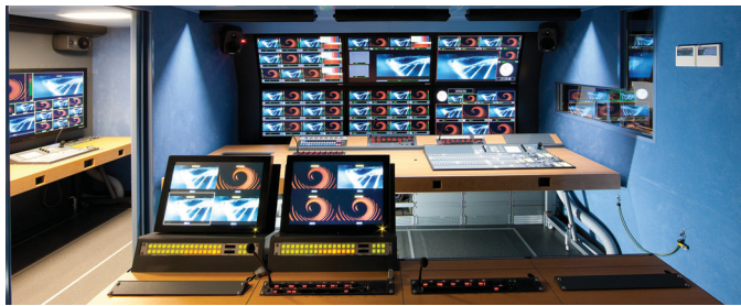
Evertz monitors and Grass Valley Kayak switcher feature in the truck's gallery, and the Lawo MC256 digital mixer, expandable to 48 faders, specified by ERR
